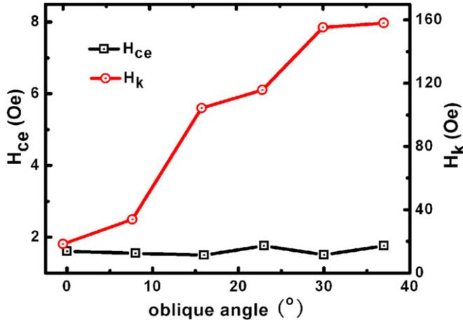
Figure 3. EA coercivity and IPUMA field  $H_k$  of  $Co_{93.5}Zr_{6.5}$  soft magnetic films as a function of oblique angle. (Colour online.)
