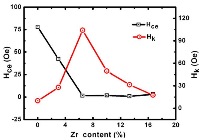
**Figure 2.** EA coercivity  $H_{ce}$  and IPUMA field  $H_k$  of Co-Zr films versus Zr concentration. All samples were deposited at  $16^\circ$ . (Colour online.)
