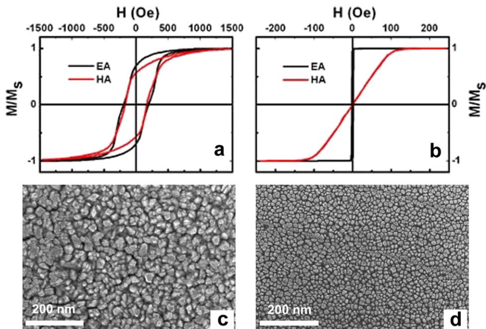
**Figure 1.** In-plane hysteresis loops ((a) and (b)) and surface images ((c) and (d)) for Co film (left column) and  $\text{Co}_{93.5}\text{Zr}_{6.5}$  film (right column). Both the samples were deposited at  $23^\circ$ . (Colour online.)
