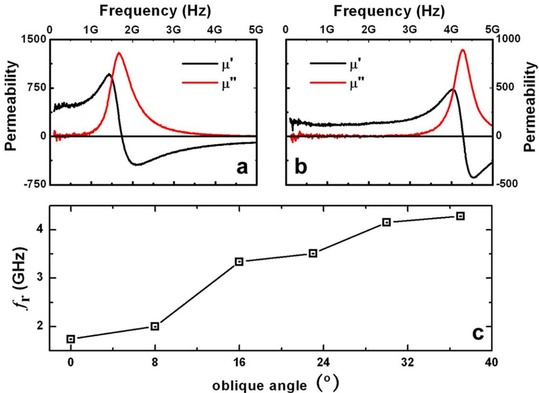
Figure 4. Frequency dependence of the relative complex permeability of  $Co_{93.5}Zr_{6.5}$  films deposited at oblique angles of ~0° (a) and ~37° (b), respectively. Oblique angle dependence of the resonance frequency of Co–Zr films (c). (Colour online.)
