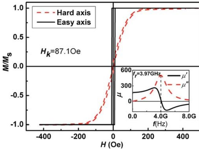
FIG. 2. (Color online) The main figure is the in-plane  $M$ - $H$  loop, where red dashed line is the  $M$ - $H$  loop of hard axis and the blank solid line is the  $M$ - $H$  loop of easy axis. The inset is the permeability spectrum of  $(\text{Co}_{96}\text{Zr}_4/\text{Cu})_{24}$  multilayers, where red dashed line and the solid line show the image part and the real part of the permeability.
