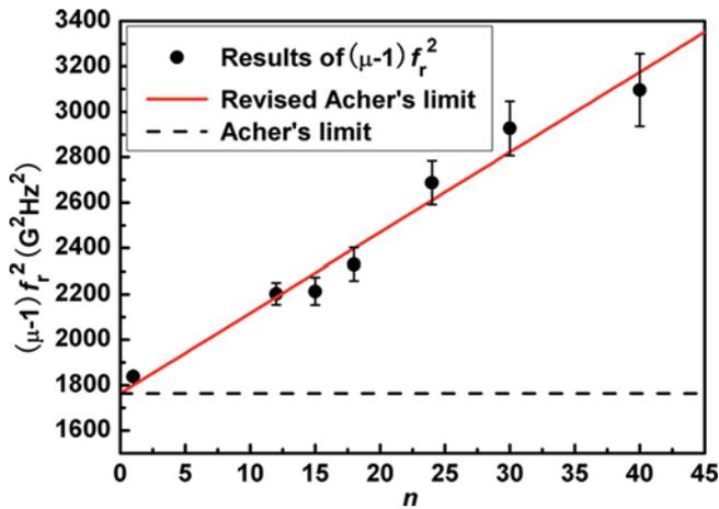
FIG. 4. (Color online) The relationship between Acher's limit and number of periods is displayed. The solid cycles are results calculated from experimental resonance frequency with function  $(\mu_s - 1)f_r^2$ , where the red solid line is fitting curve of RAL and the black dashed line is the Acher's limit of thin film.
