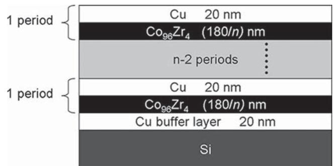
FIG. 1. The structure of  $(\text{Co}_{96}\text{Zr}_4/\text{Cu})_n$  multilayers on a 20 nm Cu buffer layer. The substrates are  $10 \times 20 \times 0.42 \text{ mm}^3$  (111)-oriented Si pieces. Thickness of each  $\text{Co}_{96}\text{Zr}_4$  layers are  $(180/n) \text{ nm}$ . Between  $\text{Co}_{96}\text{Zr}_4$  layers, there are 20 nm Cu layers to eliminate the exchange interaction.
