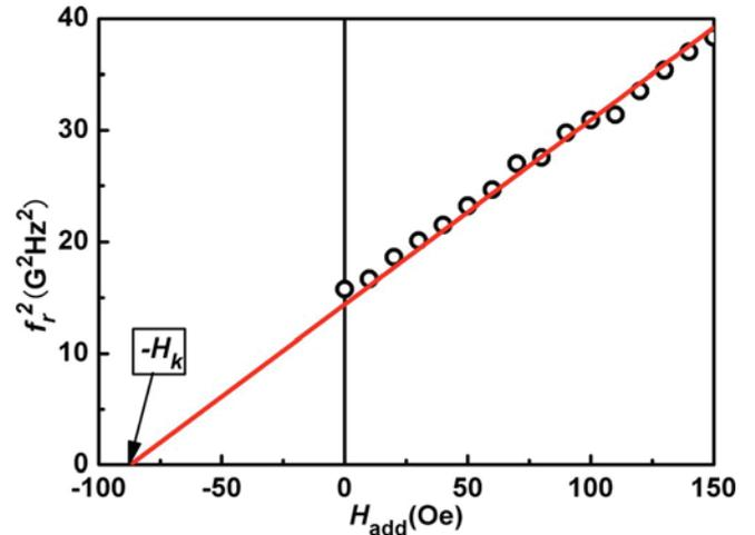
FIG. 3. (Color online) Square of the resonance frequencies for additional field  $H_{\text{add}}$  parallel to the easy axis are shown. The circles are experimental results and the red line is the fitting curve. The sample is  $(\text{Co}_{96}\text{Zr}_4/\text{Cu})_{24}$  multilayers. The value of  $H_{\text{add}}$  at the zero crossing of  $f_r^2$  is 87.0 Oe.
